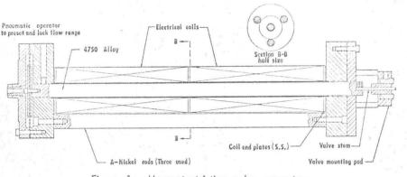
Figure 1. Magnetostriction valve operator
